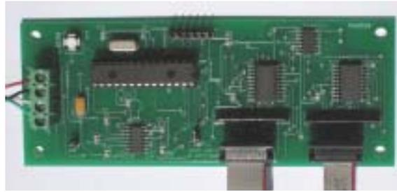
The system consists of a small pc board (shown above) and a main board. The small board mounts inside the Aiphone NHX control unit and connects to connectors CN8 and CN9. The main board is in a cabinet mounted nearby.
